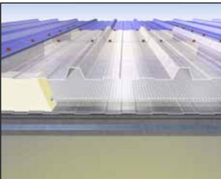
Composite panels consist of a profiled metal outer sheet and liner that are bonded on either side of a solid insulation core that allows installation by the roofing contractor as a single unit. There are through fixed systems that are installed using purpose made self-drilling fasteners and secret fix and standing seam systems that have no exposed fasteners.
