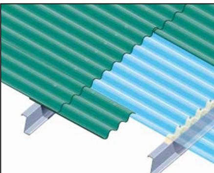
Profiled fibre cement roof systems are available with a profiled metal or fibre cement liner, spacer system, quilt insulation and a profiled fibre cement outer sheet that are assembled by the roofing contractor. Single skin systems are also available when Building Regulations allow the use of uninsulated roofs. There are through fixed systems that are installed using purpose made self-drilling fasteners. Hookbolts or similar may also be used.
