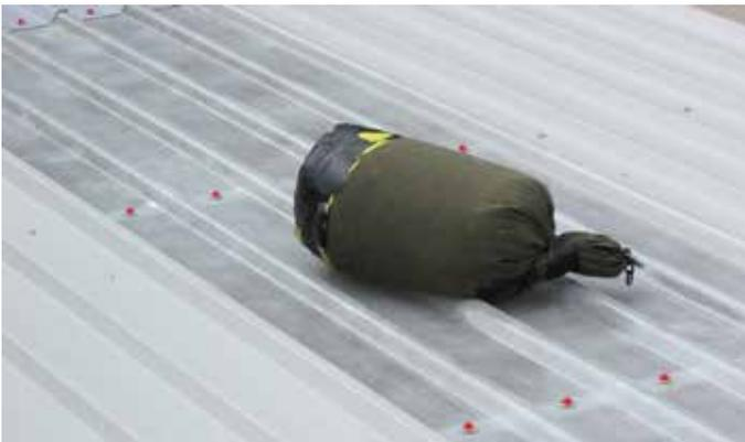
There is always the risk of trips and falls on profiled sheeted roofs. A falling person will generate an impact load on the area of roof where they land. Modern rooflight systems are designed to be impact resistant or non-fragile as defined by test to ACR[M]001, although they will often be damaged by large impacts and will require replacement. This is covered in Section 4: Non-fragility and durability.
