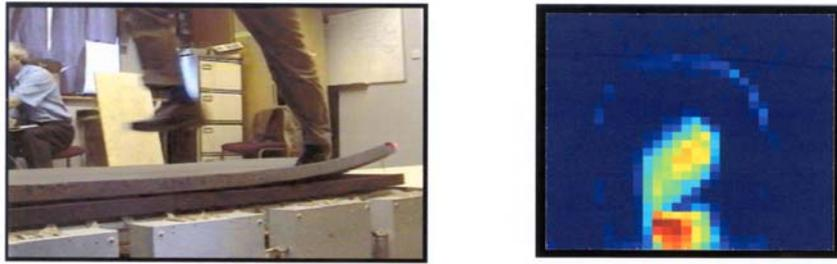
Figure 7: Video frame and pressure image of stumble event
