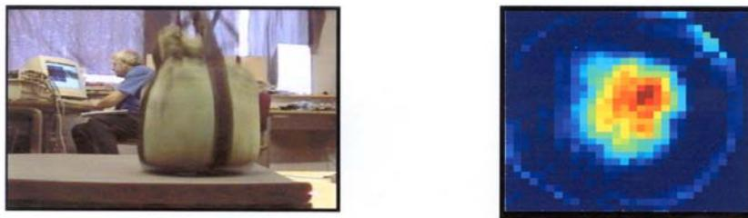
Figure 9: Video frame and pressure image of bagdrop
