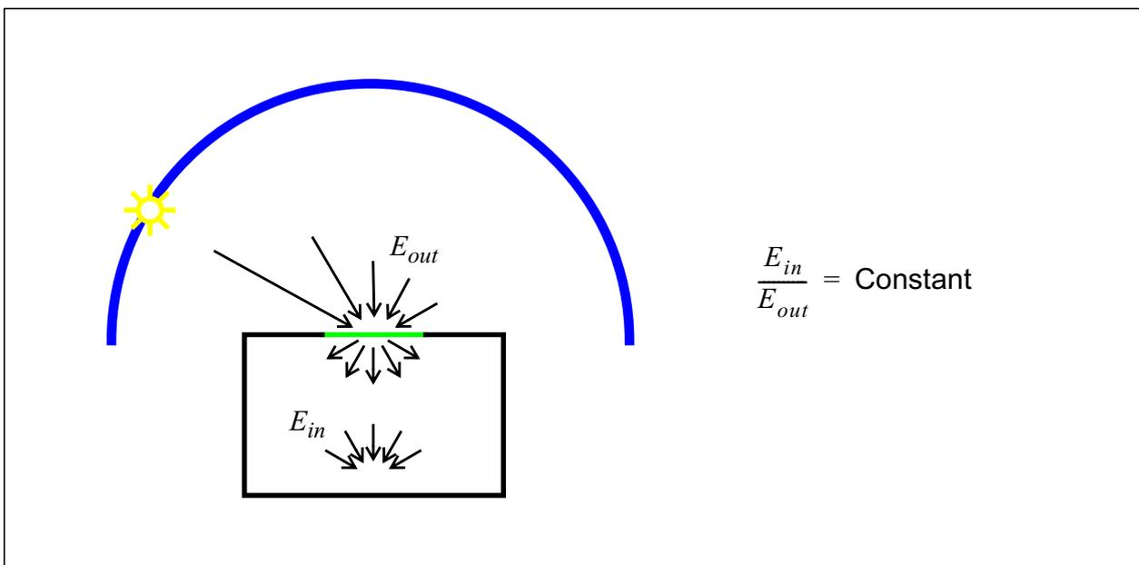
Figure 1. Constant daylight factor under horizontal diffusing rooflights
