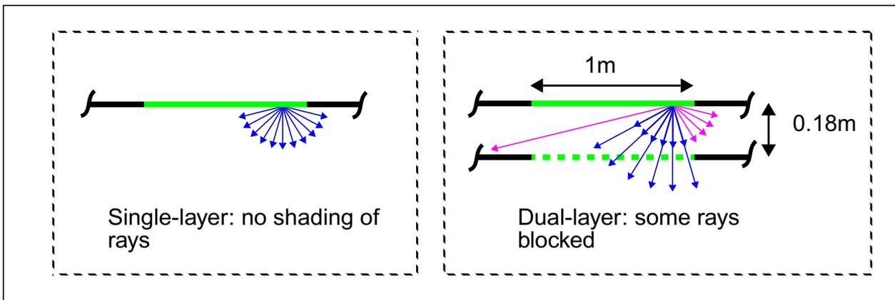
**Figure 3. Schematic showing losses to roof-void resulting from dual-layer construction.**
