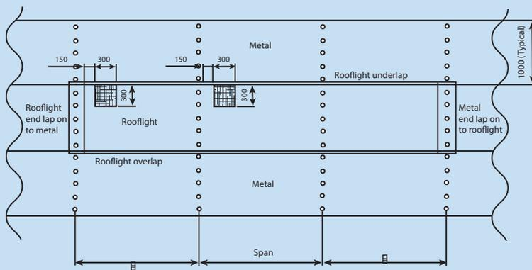
**Diagram 3. Multi-span rooflight**
