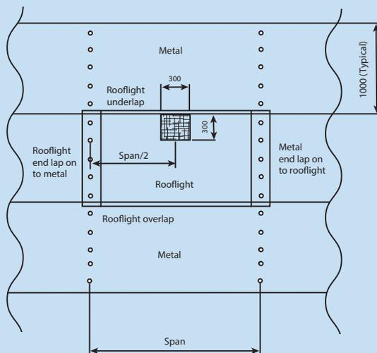
**Diagram 4. Single-span rooflight**
