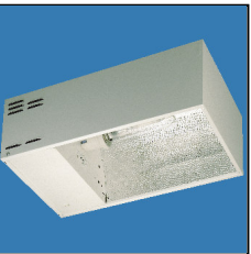
Type D Low Bay Lamps typically 250W or 400W and used at mounting height 5 m to 8 m Used in industrial areas, retail sheds
